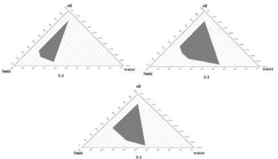
Fig 01: Pseudoternary phase diagram of tea tree oil, Tween 20, propylene glycol contains different Smix ratio (1:1, 2:1 and 3:1).
